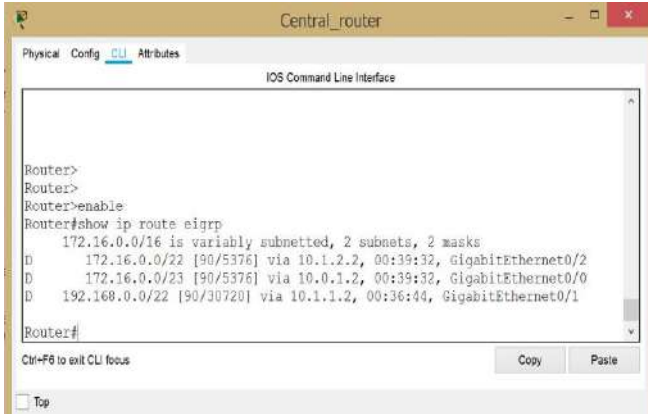
Fig. 6. Routing table of Central router in Fig. 4.
