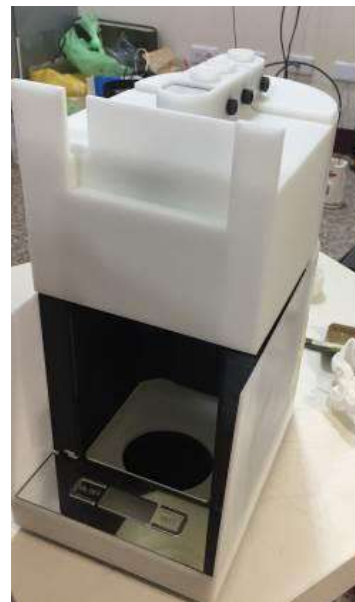
Fig. 10. Prototyping: chassis made by 3D printing.
