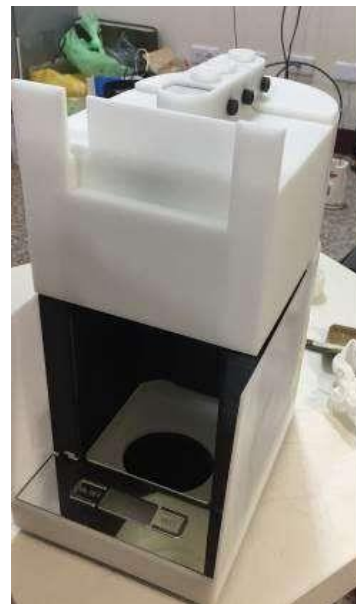
Fig. 10. Prototyping: chassis made by 3D printing.
