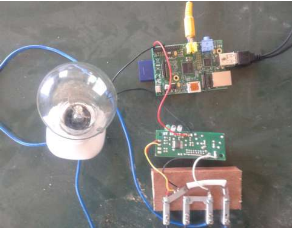
Figure 5: Load connection with proto type
