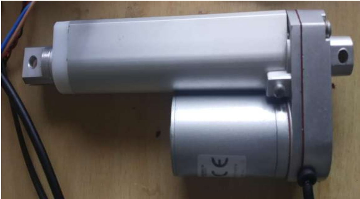
Figure 7: Actuator used for tilting the solar panel from north to south. RTC
