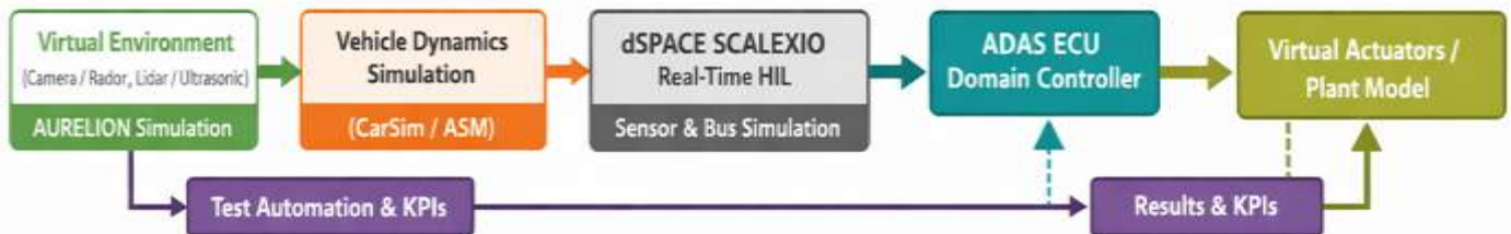
Fig. 1: HIL Simulation Framework for ADAS Testing Under Adverse Vehicle Conditions
