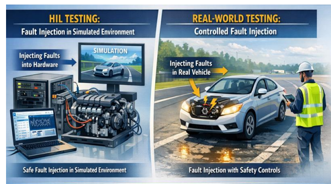
Fig. 3: Hybrid Validation through HIL and Real-World Testing
