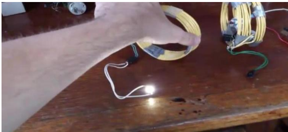
Fig. 10. Practical test for rotational misalignment.
