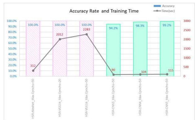
Fig. 6. Accuracy and Training time comparison of deep learning models from both strategies of “Training by using AlexNet and VGG16” and “Create new CNN from Scratch”.
