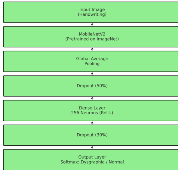
Fig. 3. Detailed Architecture of MobileNetV2-Based Model for Dysgraphia Classification
